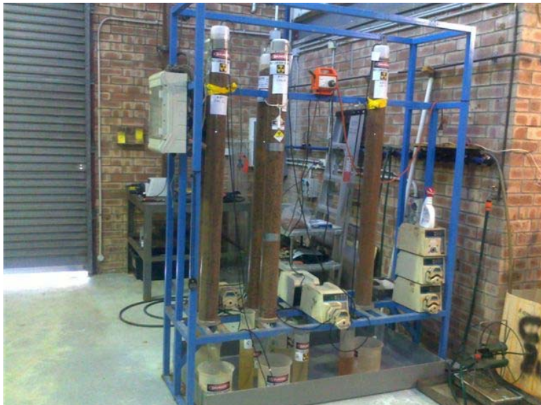
Figure 5: Column leach testwork underway at laboratory testing facility
