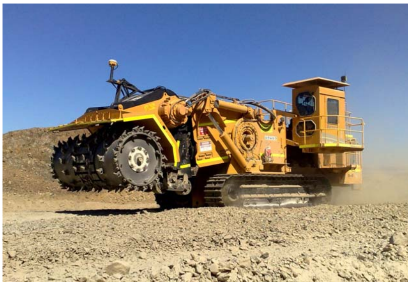
Figure 4: Resource Test Pit surface continuous miner
