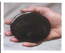
High level spent fuel product from the electricity consumption of one person's lifetime would be encapsulated in a vitrified glass disc of this size.
